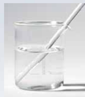
The light refraction indices of the monomer and the glass rod are different.
